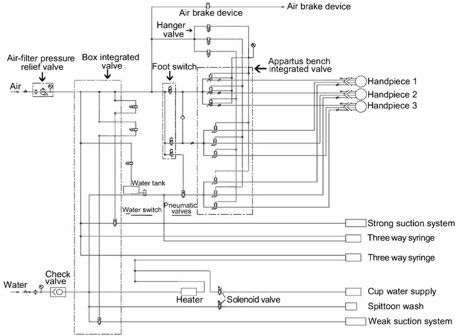
**Part 17 Schematic Diagram for Water and Air Rout**
